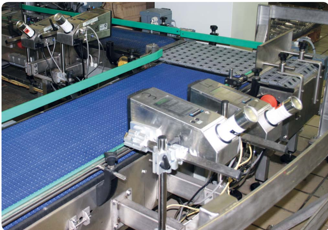
Small-footprint Videojet 2300 high resolution case coders integrated at Chavignol facility.
