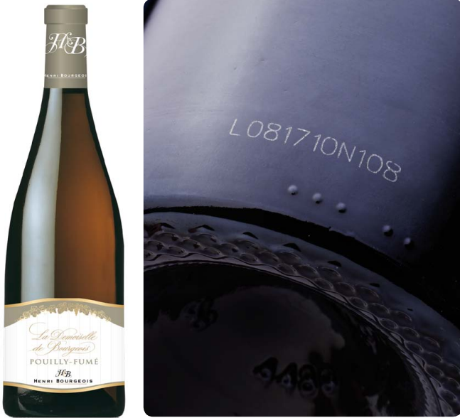
Videojet CO 2 lasers mark traceability data directly on individual wine bottles
